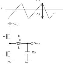
Fig.28 Output ripple current
