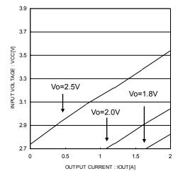
Fig.35 minimum input voltage in each output voltage
