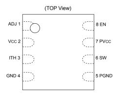
Fig.2 Pin Configuration
