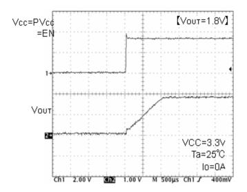
Fig.14 Soft start waveform
