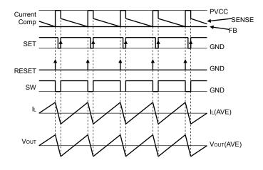
Fig.20 PWM switching timing chart
