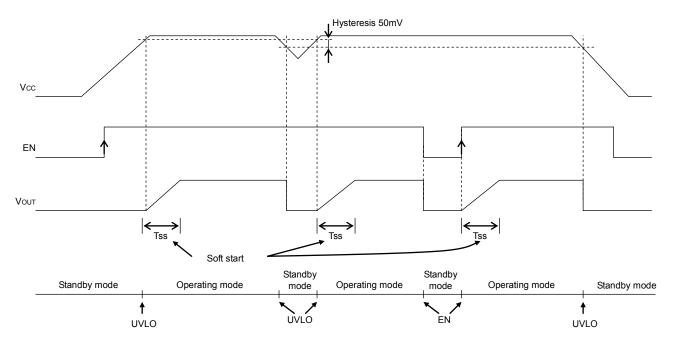
Fig.22 Soft start, Shutdown, UVLO timing chart
