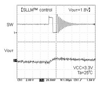
Fig.15 SW waveform Io=10mA
