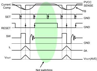
Fig.21 SLLM<sup>TM</sup> switching timing chart
