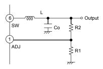
Fig.34 Determination of output voltage
