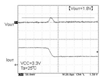
Fig.18 Transient response Io=2A→1A(10µs)
