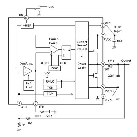
Fig.3 Block diagram
