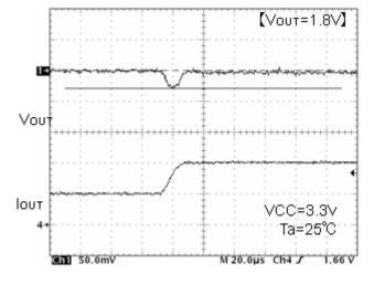
Fig.16 SW waveform Io=200mA
