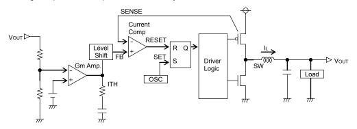
Fig.19 Diagram of current mode PWM control
