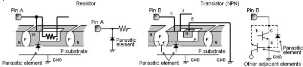
Fig.38 Simplified structure of monorisic IC
