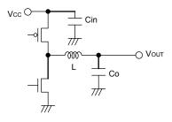
Fig.30 Input capacitor
