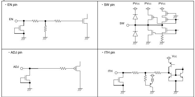
Fig.37 I/O equivalence circuit
