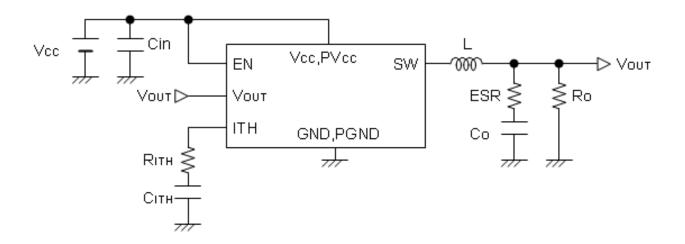
Fig.1 Typical Application Circuit
