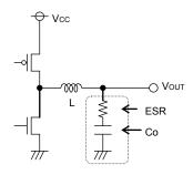
Fig.29 Output capacitor
