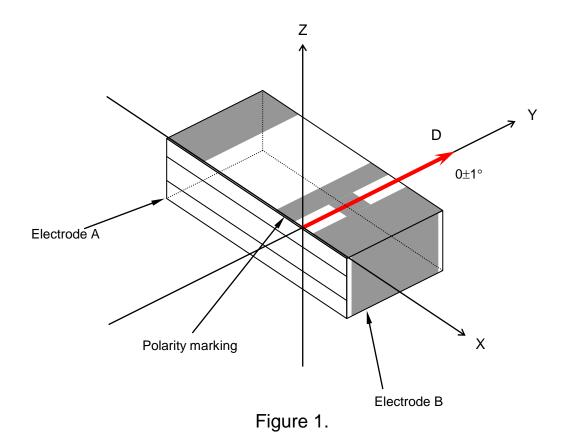
Axis D : This axis is an acceleration applied direction, when electric charge sensitivity is checked.
