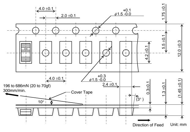
Figure.3 Dimension of Plastic Tape
