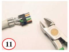
Slide load bar down to foil shields, cut wires flush
