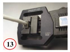
Set plug blades using Stewart Connector Crimp Tool
