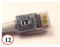
Insert load bar into plug body
