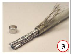
Remove cable jacket; Fold braided shield back
