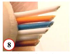
Align Org, Blu, & Brn pairs and cut ends at a 45 ° angle
