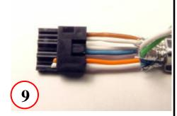
Insert Org, Blu, & Brn pairs into load bar
