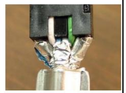
Close-up of Grn pair after being inserted into load bar
