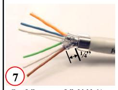
Carefully remove foil shields ¼ inch above ferrule
