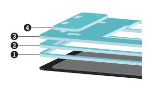
Place your Raspberry Pi 7" Touchscreen Display face down on a soft non-scratch surface and lay frames (1, 2, and 3) on top of it.
