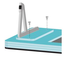
Screw in the four M3 x 6mm nylon bolts until the stands are firmly secured. Don't overtighten them!
