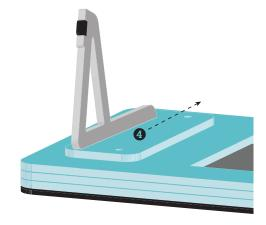
Slide the locking stand plate upwards which will align the screw holes through to the display's metal bracket.
