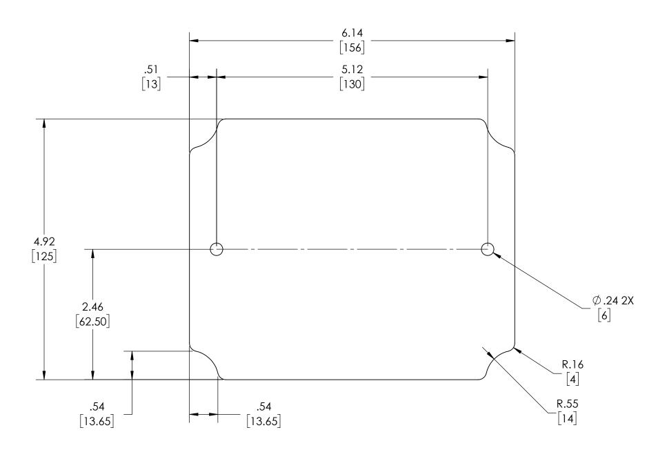
MATERIAL - .063 [1.6mm] THK. STEEL, ZINC PLATE DIMENSIONS ARE INCH[MM]
