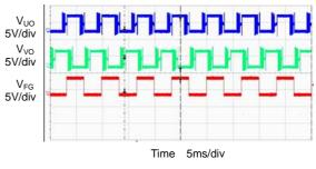
Figure 14. FG Output Signal
