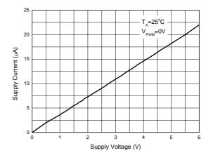
Figure 5. Supply Current vs. Supply Voltage
