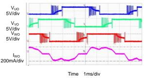
Figure 10. Rotation Mode Waveform (Forward Mode)
