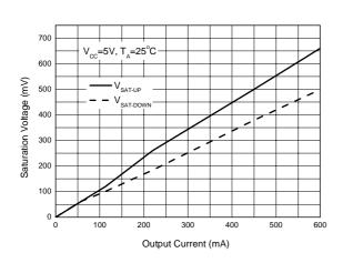
Figure 6. Saturation Voltage vs. Output Current
