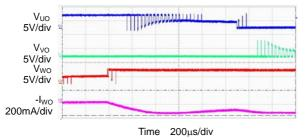
Figure 12. Soft Switching Waveform
