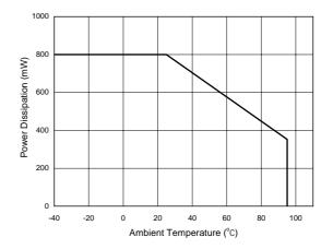
Figure 7. Power Dissipation vs. Temperature (Note 2)
