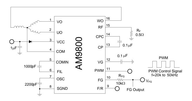
Figure 8. Typical Application of AM9800
