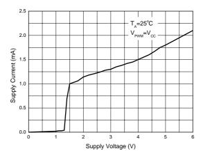
Figure 4. Supply Current vs. Supply Voltage
