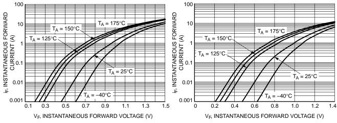
Figure 1. Typical Instantaneous Forward Characteristics
