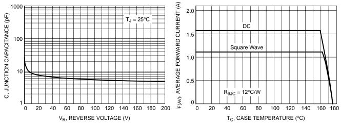
Figure 5. Typical Junction Capacitance
