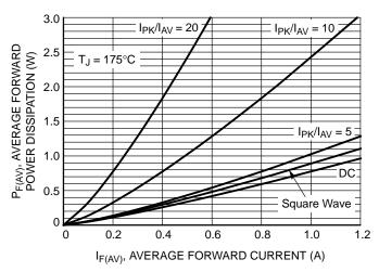
Figure 7. Forward Power Dissipation
