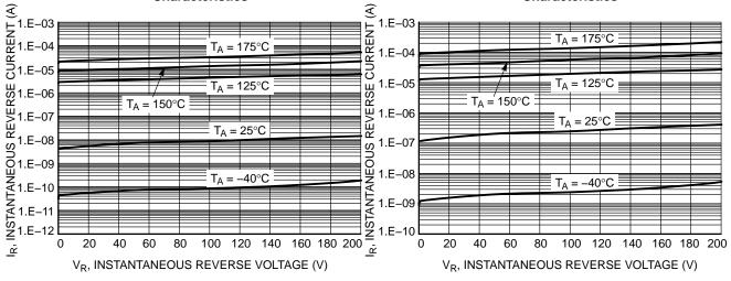
Figure 3. Typical Reverse Characteristics
