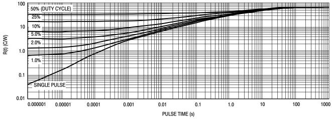
Figure 9. Thermal Response, Junction-to-Ambient (1 in<sup>2</sup> pad)
