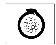
Figure A-4.1 Preferred Insulation Crimp
