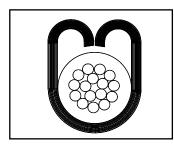
Figure A-4.4 Marginal Insulation Crimp
