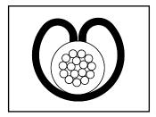
Figure A-4.3 Marginal Insulation Crimp
