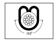
Figure A-4.2 Acceptable Insulation Crimp
