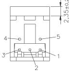
PIN FUCTION: 1.GND 2.Vcc 3.Vin 4.NC 5.NC
