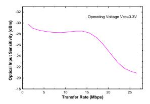
Note: Before using the EAPLRAA4 device, please confirm the minimum sensitivity at different operating voltage and transmission rate.
