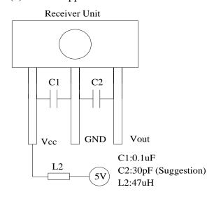
Note: For having good coupling, the C1,C2 capacitor must be placed within 7mm
