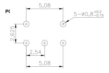
Note: PCB Tolerances:1.6mm. Unit = mm
